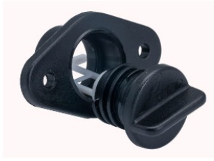
Figure 11 - Hull drain fittings old (bayonet) & new (screw).
