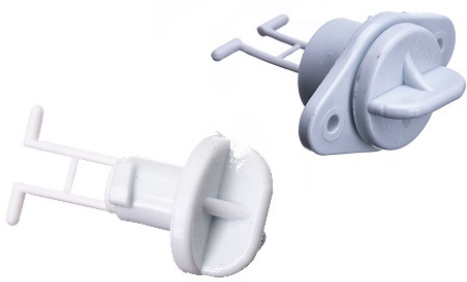
Figure 11 - Hull drain fittings old (bayonet) & new (screw).
